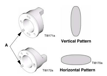
Fig. 11: Position Air Cap
